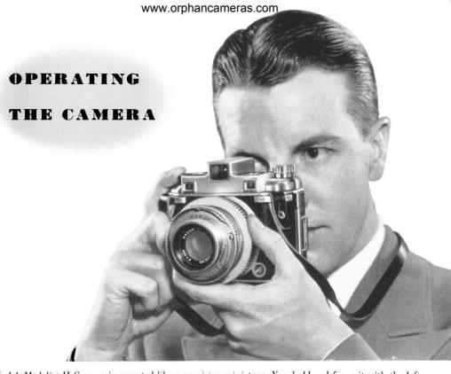
Kodak Medalist II Camera is operated like a precision miniature. You hold and focus it with the left hand ... check composition and focus through the twin view- and range-finder eyepiece (see below). The right hand advances roll film, automatically cocking the shutter (or changes film holders, pulls film-pack tabs, and cocks the shutter with the rear lever) ... then operates the body plunger release.
